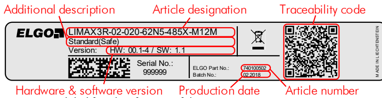
Fig. 2: Type label for identification of the sensor
