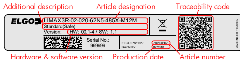
Fig. 2: Type label for identification of the sensor
