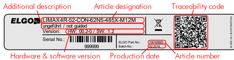
Fig. 3: Type label for identification of the sensor
