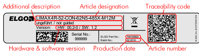
Fig. 3: Type label for identification of the sensor
